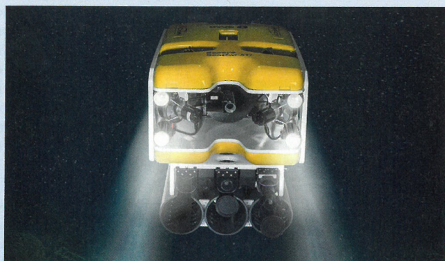
MuMNS is based on a number of mine neutralisation disruptors carried by a highly manoeuvrable Remotely Operated Vehicle (ROV). (Photo: Courtesy of Saab Group)
