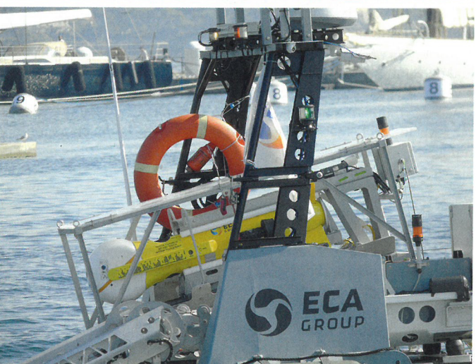
ECA Group's waterjet-powered INSPECTOR Mk2 is a commercial boat-based USV that can be equipped with LARS for launching AUVs like SEASCAN Mk2 (top), K-STER (below), and A-9M. (Photos: Courtesy of Victor M.S. Barreira)
